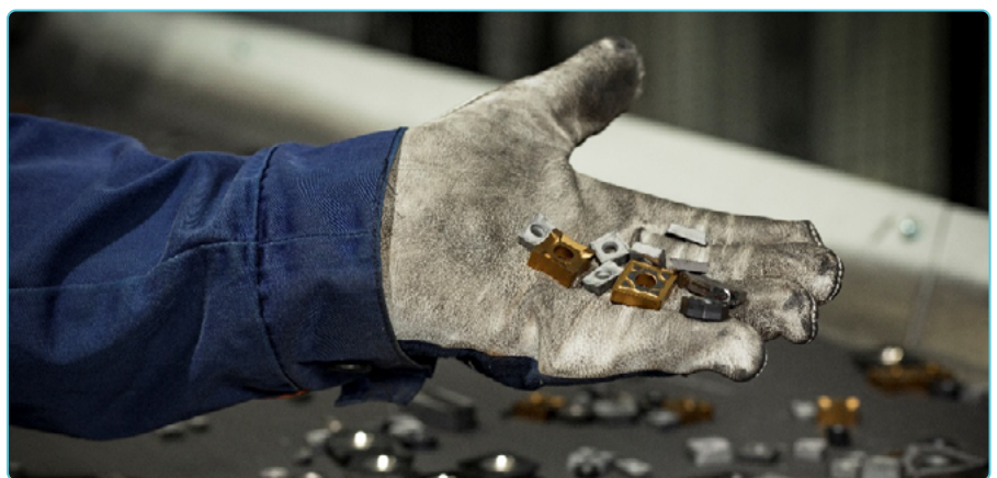
Figure 6 | Left: Dust exposure is one of the key aspects of treating hardmetal; Right: Typical mix of end-of-life hardmetal tools, with coated and uncoated grades, different shapes and size
