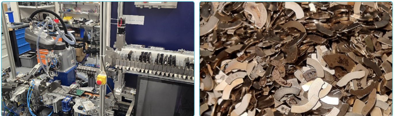
Figure 25 | Left: Robotized disassembly unit for 3,5" HDD (left); Right: Recovered and segregated NdFeB magnets from HDDs (right)
