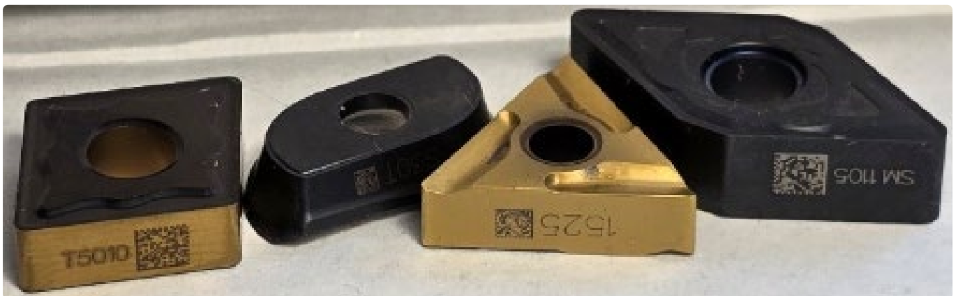
Figure 5 | Examples of various insert geometries with good quality codes.
