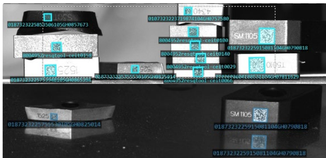
Figure 6 | Sample results of codes reading from inserts with use of developed algorithms and setups on different surfaces and code types.
